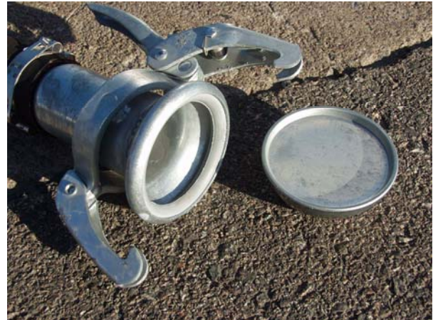
Picture 5c: Shore side coupling to be placed at berth for connection to sludgetruck
