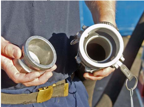
Picture 5b: Ship side connection 2 1/2" quickcoupling (camlock)
